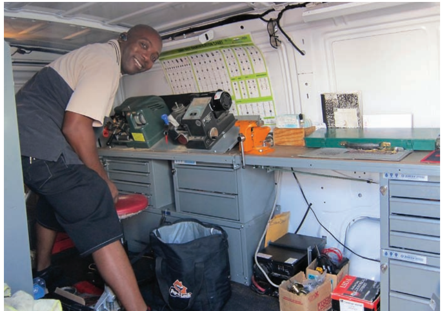
Pop-A-Lock’s low-profile 2005 Chevy Astro is outfitted with an HPC 1200 Blitz Code Machine, duplicator machine, transponder programmers and high-security key machine. Locksmith Bobby Colbert calls the van the “most organized locksmith vehicle in the USA.”
